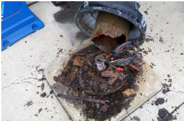
Rust and corrosion inside of a pole.
